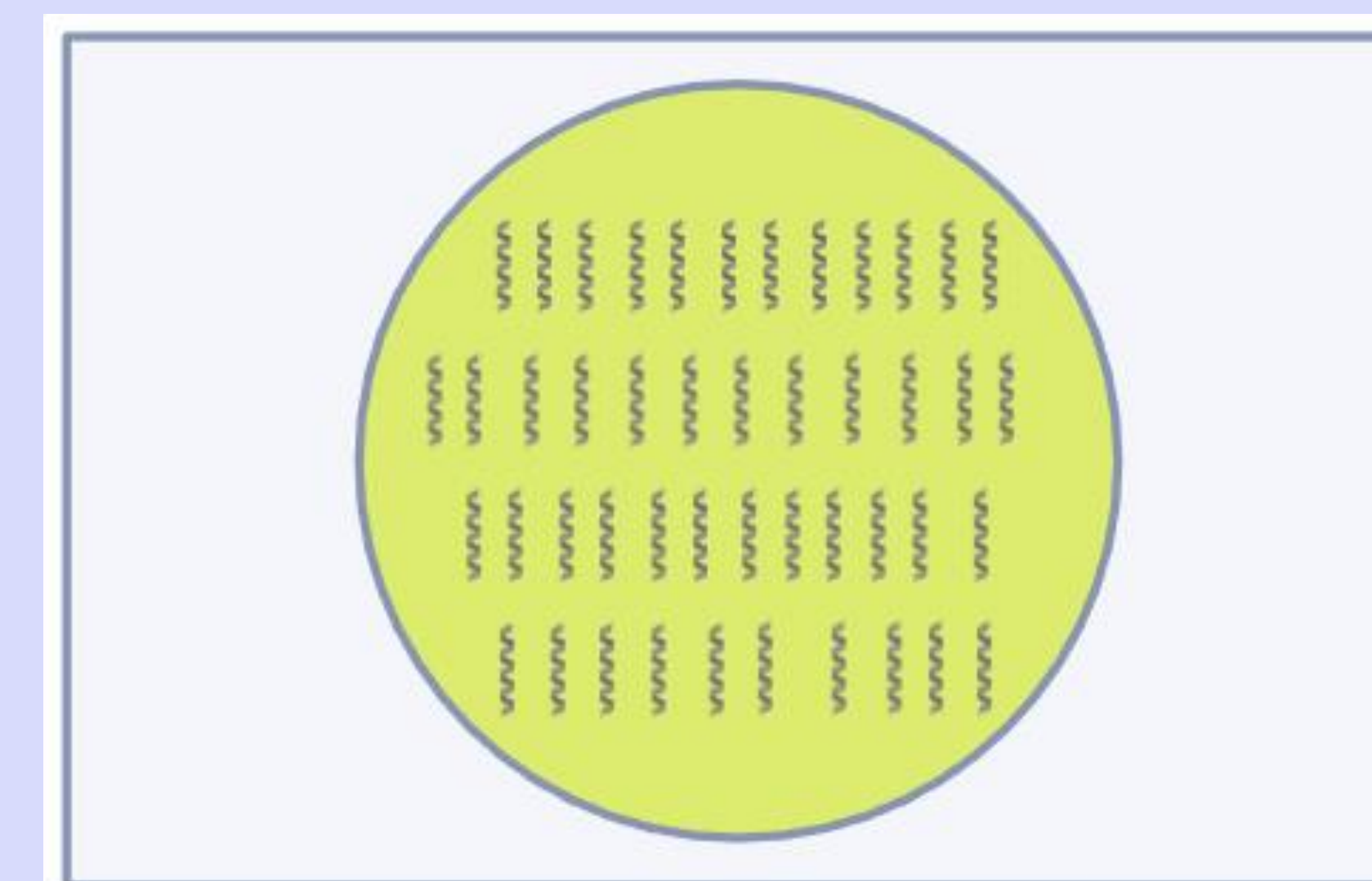
Visual representation of one layer of the helices suspended in the resin after 3D printing (not to scale).
